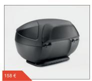
Top box with 39L storage, including backrest. 1-key operation requires cylinder inner kit (08885-HAC-P00) and cylinder body kit (08885-HAC-P10). Rear carrier (08L00-MGZ-RTB) is required to fit this accessory.
