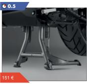
Main stand ensures secure parking on variable surfaces and facilitates chain maintenance and rear wheel cleaning.
