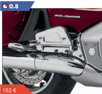
Chrome-plated injection-moulded ABS plastic construction; add stylish detail to underside of the pillion floorboards when folded and not in use.
