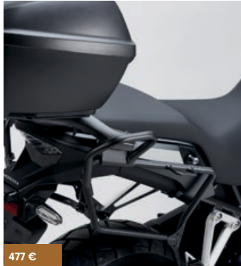
PANNIERS STAY 08L74-MKP-J80ZA Robust mounting system for the Plastic Panniers Set.
