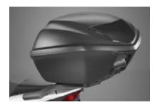
35L TOP BOX KIT DBESY-KIZ-35TB 35-liftres plastic Top Box with a backrest that can store 1 helmet. Top box base and key system included. 227 €
