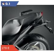
Replacement seat maintains comfort while improving ground reach; +/- 28mm lower and +/- 14mm narrower than standard.
