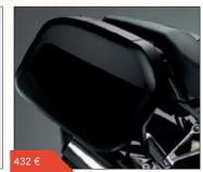
Rear panniers designed to complement the CB500F's style; 1-key cylinder (08M71-KZL-840), lock assembly (08L00-KZL-860) and pannier stay kit (08L74-MGZ-J00ZA) are required to fit this accessory.
