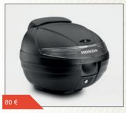
29L top box includes pillion backrest. 1-key operation requires addition of cylinder inner kit (08885-HAC-P00) and cylinder body kit (08885-HAC-P10). Rear carrier (08L00-MGZ-RTB), stay assembly right carrier (81203-MGZ-D00) and stay assembly left carrier (81204-MGZ-D00) are required to fit this accessory.
