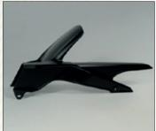
Protects the shock absorber from road grime and water, with integrated chain guard.
