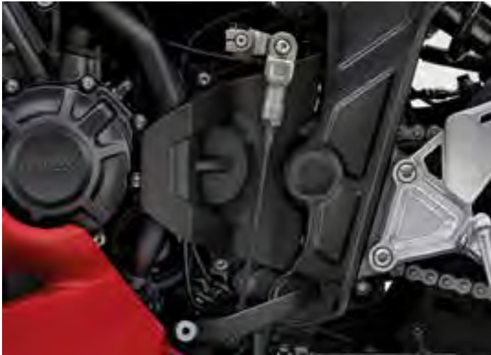
QUICK SHIFTER KIT 08U72-MKN-D50 By measuring the intensity of the shifting input, the quick shifter enables the rider to change gear without the need to operate the clutch lever or shut the throttle. The system aids upshifting, maximizing the riding experience. Not compatible with E-Clutch versions.
