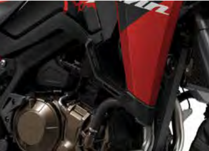
DEFLECTORS SET 08R72-MKS-E00 The deflectors improve comfort by reducing travelling air around the rider's waist and knees while funnelling the warm air emitted by the radiators.
